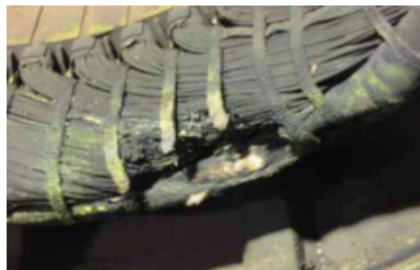
变频器对定子绕组的损伤 The damage of inverter to stator winding
